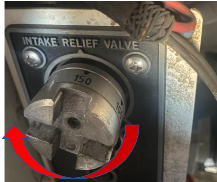
Figure 21: Rotate the intake relief valve in a clockwise motion to increase intake GPMs
