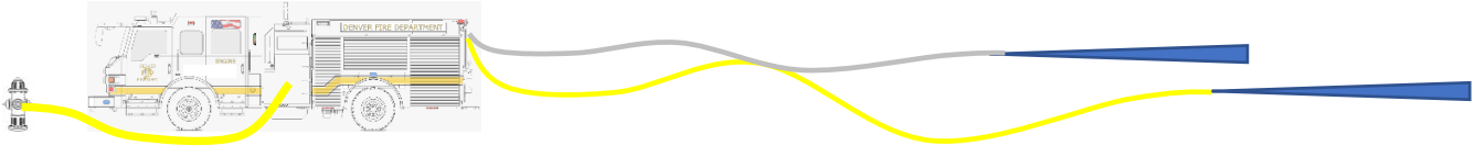
Figure 12: 300' of 2-1/2" Hoseline with a 1-3/16" Smooth Bore Nozzle with a Target Flow of 300 GPM and a 200' 1-3/4" Hoseline with a 15/16" Smooth Bore Nozzle with a Target Flow of 180 GPM
