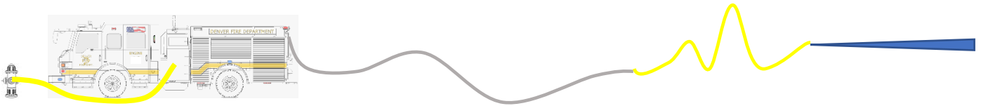
Figure 5: 200' of 1-3/4" Hoseline Extended with a 50' Section of 2-1/2" High Rise Hose with a 1-3/16" Nozzle Flowing 300 GPM
