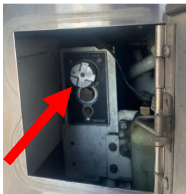
Figure 20: The intake relief valve is typically located on the Officer's side pump panel
