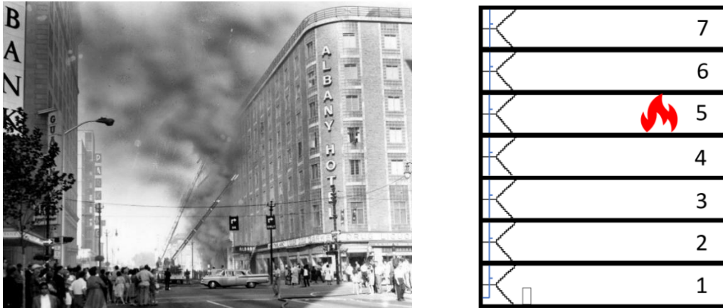
Figure 4: Pump to a 7-Story Standpipe Equipped Building with a Fire on the Fifth Floor Copyright https://history.denverlibrary.org/news/albany-hotel-fire
