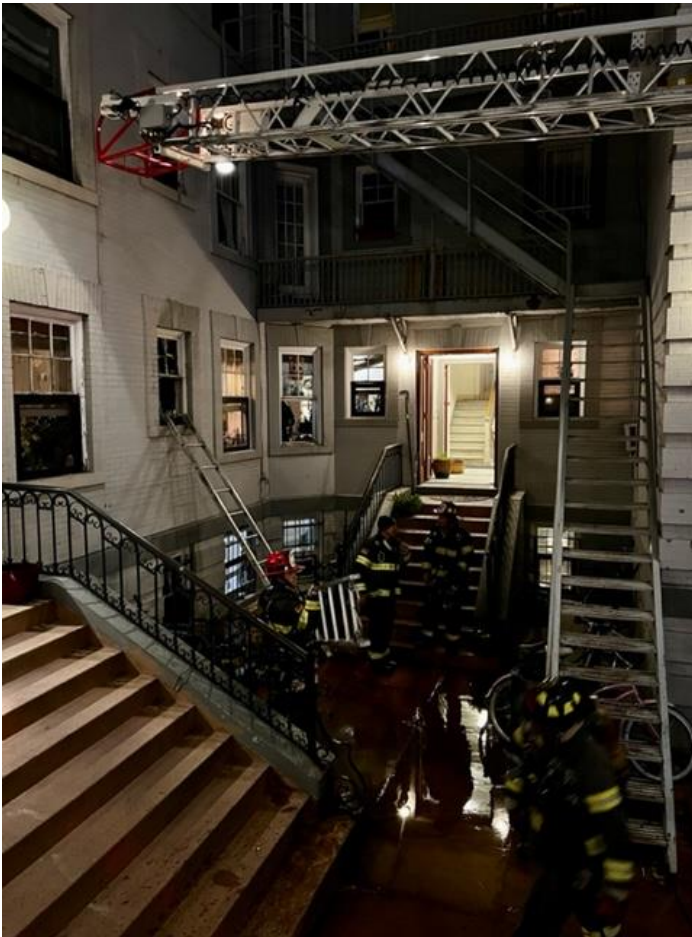
Figure 17: Courtyard placement of an aerial (T8)
